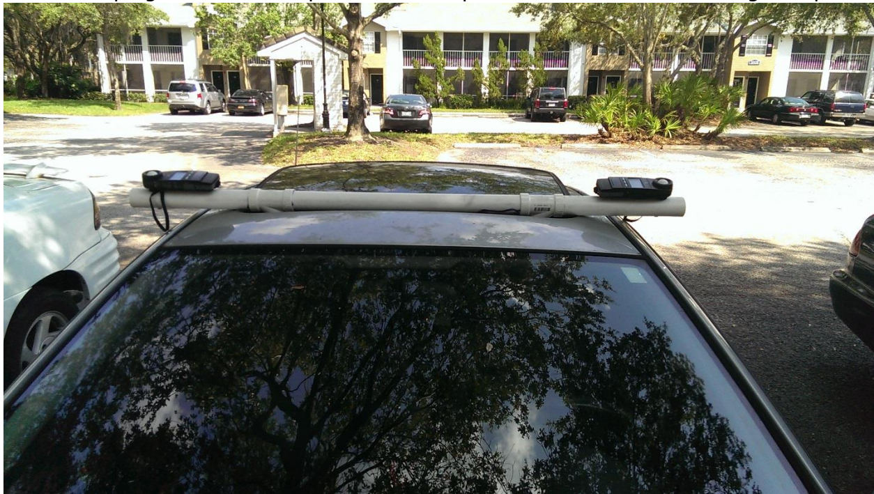
Figure 17: Light meters mounted on top of vehicle
